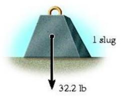
Hence, a body of mass 1 kg has a weight of 9.81 N, a 2 kg body weighs 19.62 N
